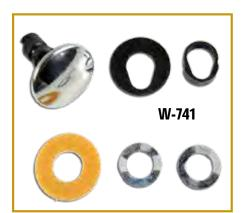
FAITHFUL REPRODUCTION VENT WINDOW PIVOT STUD (6) PIECE ASSEMBLY (W-741) FEATURES AN EXTERIOR HIGH POLISH STAINLESS BUTTON CAP, INNER FIBER AND OUTER RUBBER SEALS, INTERNAL PLASTIC BUSHING SPACER AND TWO SPECIAL WAVE WASHERS (ONE EXTRA). COMPLETE KIT (W-733) INCLUDES TWO STUD ASSEMBLY, TWO NICELY CHROME PLATED RETAINER NUTS AND RH AND LH HANDLES WITH INCLUDED ROLL PINS (18 PIECES). DOES BOTH RH AND LH VENT WINDOW GLASS. ALL PARTS AVAILABLE SEPARATELY. PACKAGED WITH A COLOR LOGO HEADER CARD.
